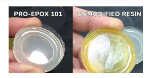
is, extra work, extra time until full cure and loss of the recoat window. Hence, a resin system which minimizes or eliminates blushing is a significant aid when working in the yard.
